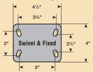
TSG/TFG top plates are 1/4" thick and have fixing holes to suit 3/8" diameter bolts.
