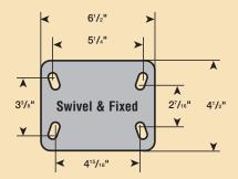
Alternative top plates are 1/4" thick and have fixing holes to suit 3/8" diameter bolts. To order, contact factory.
