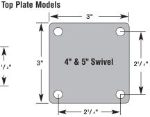
TSED 100 & 125 top plates have fixing holes to fit 5/16" diameter bolts.
