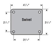
Top plates have fixing holes to suit 5/16" diameter bolts.
