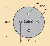
2SL top plates have fixing holes to suit 1/4" diameter countersink head screws.
