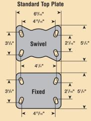
XSH/XFH top plates have fixing holes to suit 1/2" diameter bolts.
