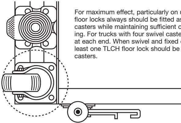
For maximum effect, particularly on uneven floors, TLCH Series floor locks always should be fitted as close as possible to swivel casters while maintaining sufficient clearance (radius) for swiveling. For trucks with four swivel casters, use one TLCH floor lock at each end. When swivel and fixed casters are used together, at least one TLCH floor lock should be used next to the swivel casters.
