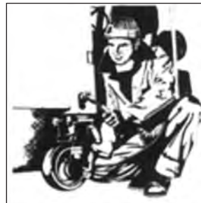
5. Tighten locking screw using ratchet spanner
