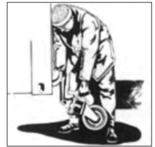
2. Attach handle and lift caster
