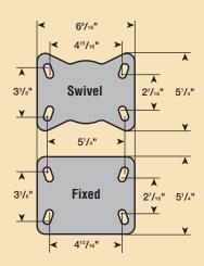
RSH & MSH swivel top plates are 9/32" thick and have fixing holes to suit 1/2" diameter bolts.
