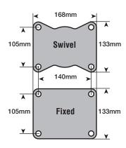
T05 top plates have fixing holes to suit 12mm diameter bolts. To order, add suffix **T05** to Swivel or Fixed Part #
