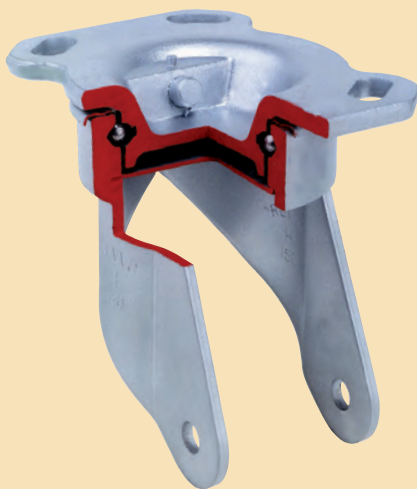
H Series casters feature a full ballrace of 2-3/8" diameter with steel ball bearings in hardened raceways sealed against contamination.
