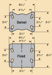
2SH swivel top plates are 9/32" thick and have fixing holes to suit 1/2" diameter bolts.
